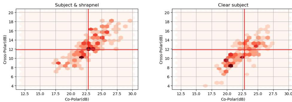
Figure 4. Distribution of reflected radar power for a subject with (left) and without (right) metallic shrapnel. Red lines indicate the average cross-section across both data sets (with and without shrapnel). It can be seen that the presence of the shrapnel changes the relationship between the cross and co-polar cross section.
