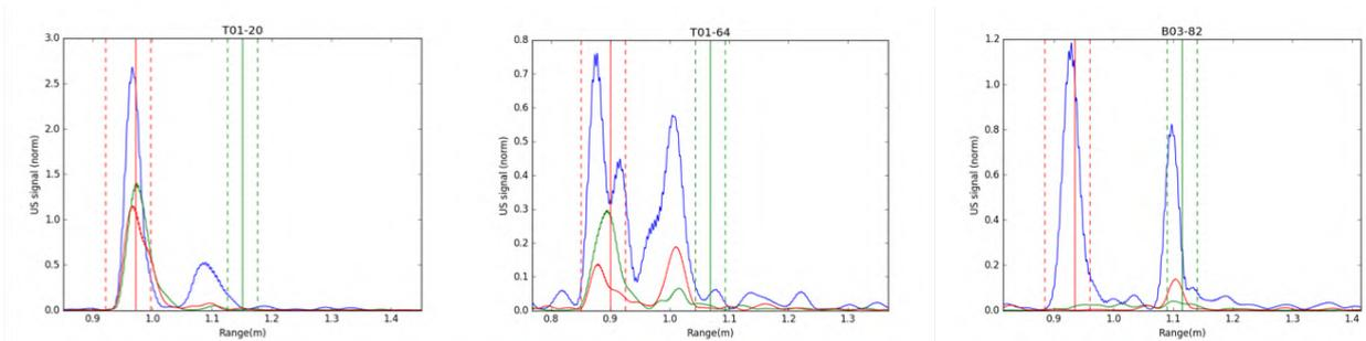
Figure 5. Ultrasound reflections from bags with different contents: plastic explosive simulant, powder explosive simulant and a mostly-empty bag (left to right). Note change in vertical scale between graphs. Each colour represents a different frequency of ultrasound (blue = 20 kHz, red = 30 kHz and green = 40 kHz).
