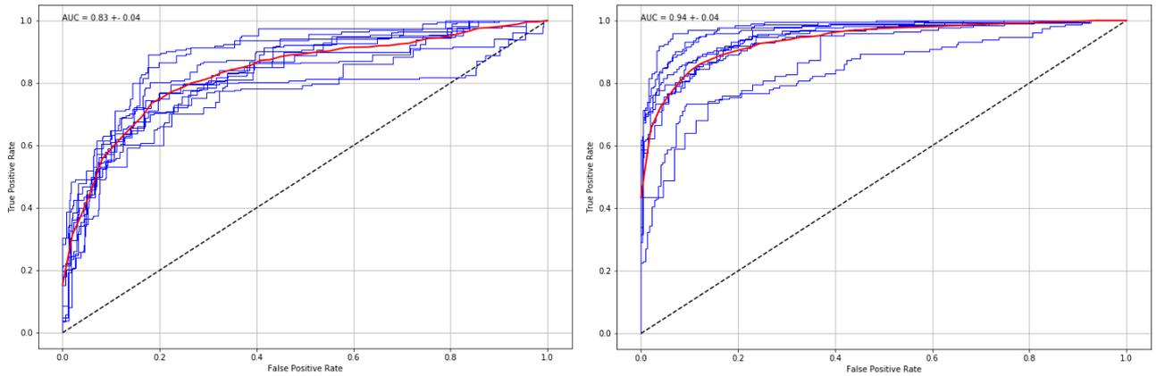
Figure 8. Receiver operating characteristic (ROC) curves for system performance on unseen data for subjects carrying either benign or threat bags (left) and subjects without bags or with person-borne threats (right). Each blue curve is performance on a specific hold-out set and the red curves represent the average of 10 different hold-out sets.
