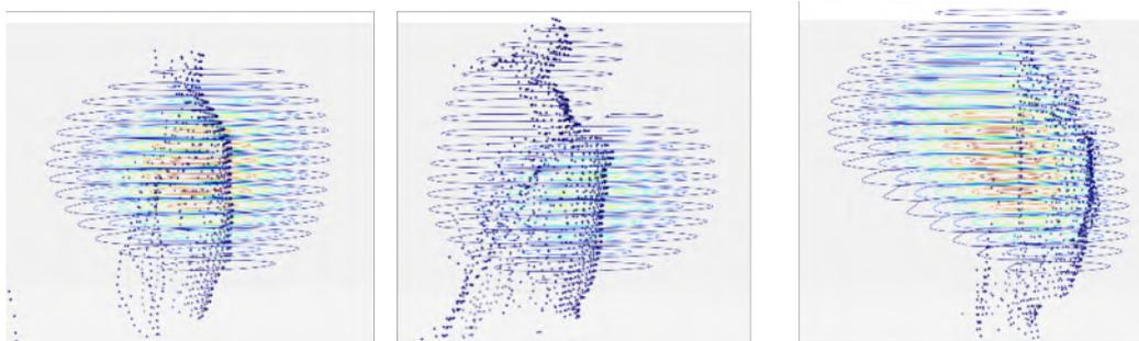
Figure 2. 3D radar images returned from subjects without a threat, wearing a pipe-bomb vest and carrying a plastic explosive simulant in a bag(left to right). The radar propagates from the right of each image. Dotted marks indicate the position of the subject, as shown by the 3D camera. The apparent shift in position of the explosive threat is due to propagation delays through the dielectric material.
