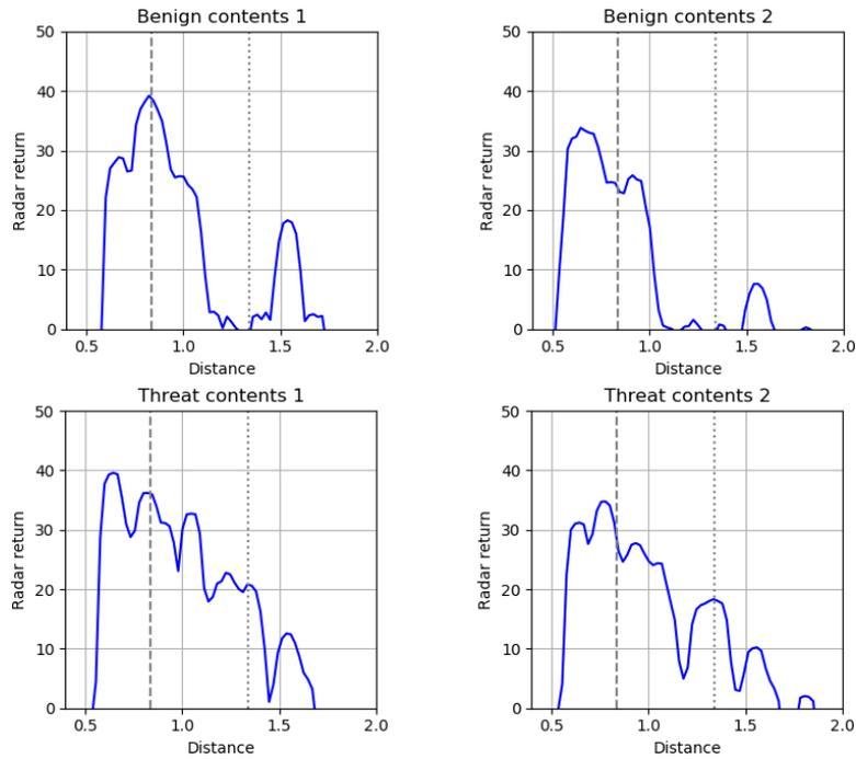
Figure 3. Millimetre-wave FMCW radar returns (using original 60 GHz radar) from two benign bags (top row) and two threat bags (bottom row). Approximate position of the back of the subject’s torso is illustrated with a dashed line.
