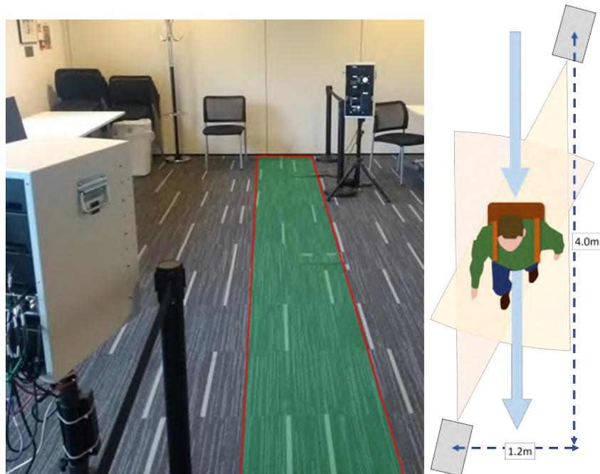
Figure 7. Photo of system set-up with walking path highlighted in green (left) and diagram of this preferred layout showing a person being screened (right).
