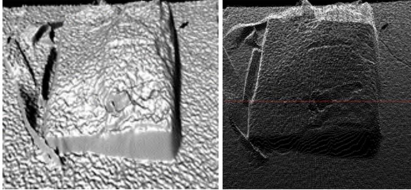
Figure 1. Time-of-flight images of a satchel on a flat surface captured by the Kinect One. The left image shows a single exposure (surface map), while the right image is an average of multiple exposures (point cloud).
