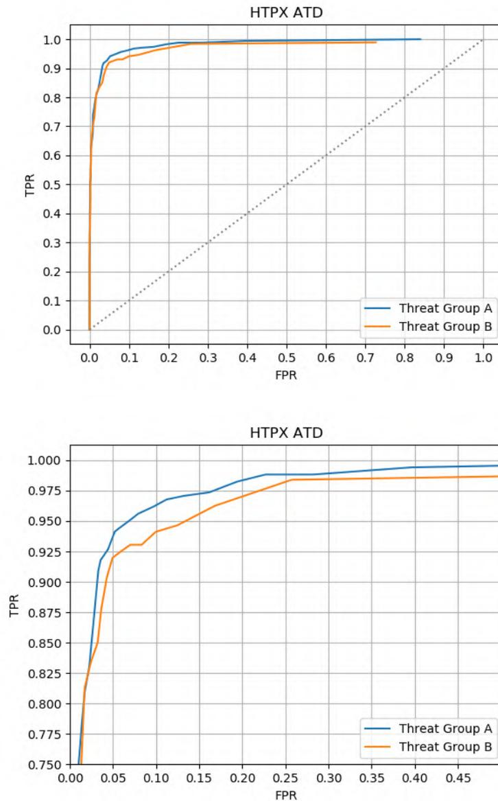
Figure 4. ROC curves using the final algorithm for different subsets of threat item on a random sample of 1,500 bags screened during a data collection trial at a London visitor attraction. Threat group A consists of the larger firearms and IEDs, group B includes medium-sized threats. Bottom image shows a close-up of the top left-hand region.
