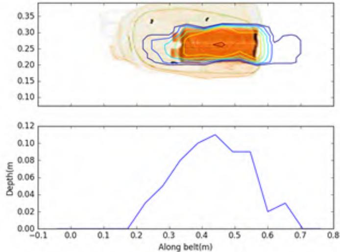
Figure 2. Radar image of a bag containing two 1 litre bottles of water. The top image shows reflected radar energy overlaid on the X-ray image. The bottom graph shows the corresponding radar measurement of average depth along the length of the bag.
