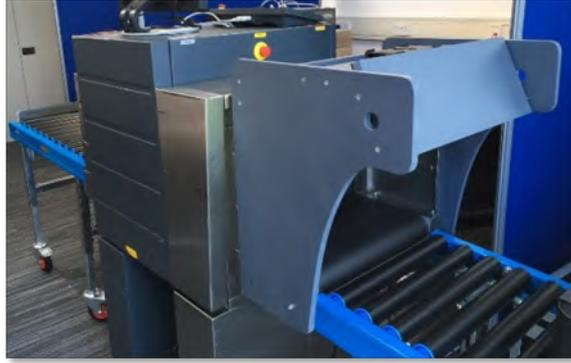
Figure 3. The HTPX proof-of-concept prototype showing X-ray machine with a hood containing the additional sensors.
